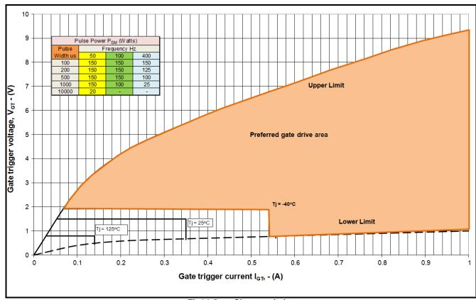
Fig14 Gate Characteristics
