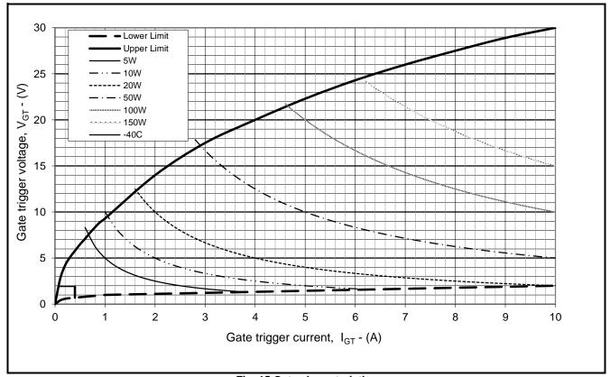
Fig. 15 Gate characteristics
