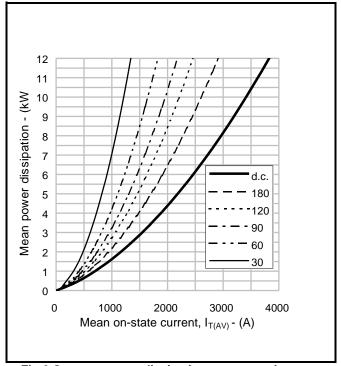
Fig.6 On-state power dissipation - rectangular wave
