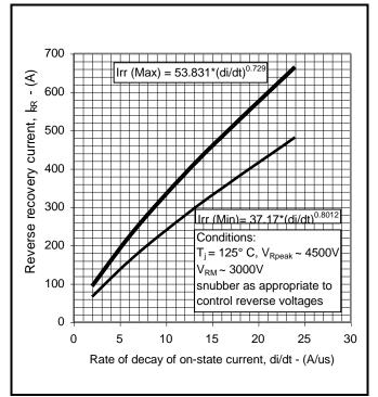
Fig.13 Reverse recovery current
