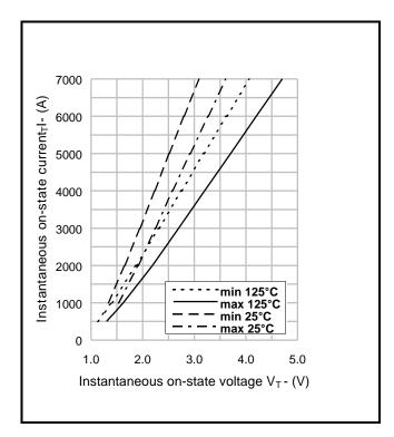
Fig.2 Maximum & minimum on-state characteristics
