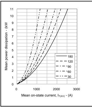
Fig.3 On-state power dissipation - sine wave
